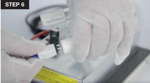
6. While holding the porcelain end-cap (with 4 pins), carefully push the white connector onto the four pins. The plug is designed so that it can only be installed one way. You may have to rotate the socket 90° to line up the pins with the holes. The connector will fit into position.
