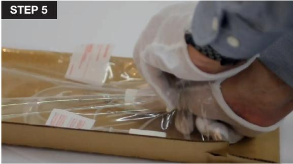
5. Carefully slide the new **UV lamp** out from the cardboard sleeve. Be sure to wear the **cotton gloves** (included) guaranteeing a clean lamp free from fingerprints. Fingerprints on the lamp will negatively impact the UV output of the lamp.
