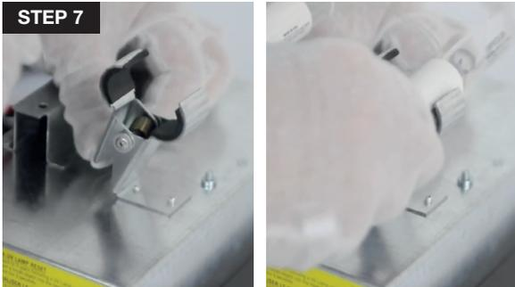
7. Slide the **UV lamp porcelain end-cap (with 4 pins)** through the clamp. Once the UV lamp is inserted, release the clamp to fix the lamp in place.
