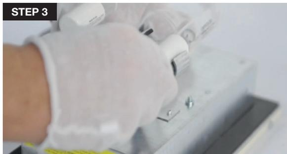
3. Remove the old UV lamp from the lamp socket by opening the retaining clamp and pulling the UV lamp out.
