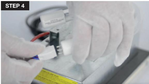
4. While holding the porcelain end-cap (with 4 pins), carefully push the white connector onto the four pins. The plug is designed so that it can only be installed one way. You may have to rotate the socket 90° to line up the pins with the holes. The connector will fit into position.
