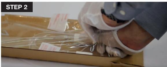
2. Carefully slide the **UV lamp** out from the cardboard sleeve. Be sure to wear the **cotton gloves** (included) guaranteeing a clean lamp free from fingerprints.
