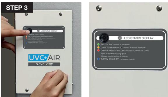
3. First turn ON the power switch and then, press the reset button. You have 5 seconds from the moment the unit is powered to press the reset button to activate the airflow detection. Every time you press the button you will notice that the LED color will either be “Blue” or “White”. Once the LED is “Blue”, wait 5 seconds while holding the reset button for the control circuit to save the setting.
