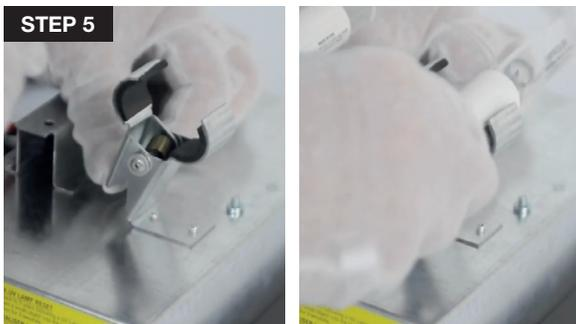
5. Slide the **UV lamp porcelain end-cap (with 4 pins)** through the clamp. Once the UV lamp is inserted, release the clamp to fix the lamp in place.
