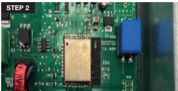
2. Plug in the UVC+ AIR to a power source and turn ON the unit by pressing the power button. In the first 5 seconds from powering the unit ON, click the Reset button once. By doing so, you'll see the status LED turn Blue meaning the airflow detection is activated. By clicking again within 5 seconds, LED will turn White meaning that airflow detection is deactivated.
